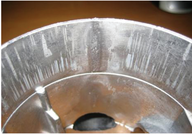
Figure 8 – Untreated Core Pin – 250 parts. (Courtesy of Long Minh Huynh-DST Technologies Pty, Ltd)
