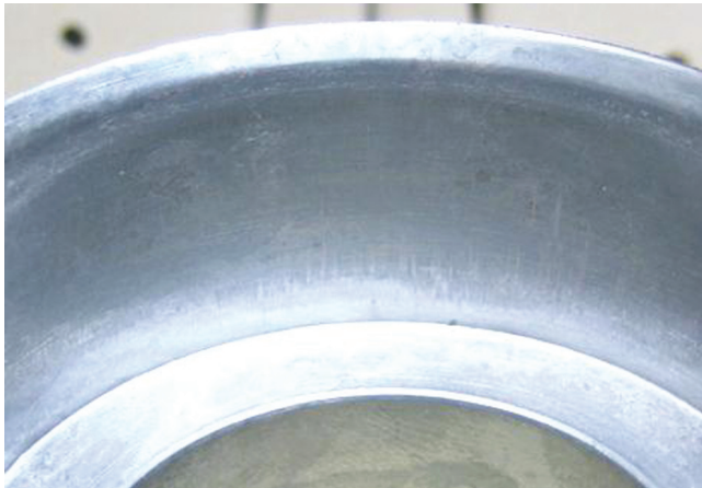
Figure 9 – DST-Cr Core Pin – 30,000 parts. (Courtesy of Long Minh Huynh-DST Technologies Pty, Ltd)
